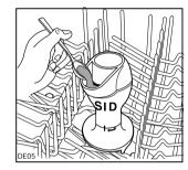
All the programmes with a warm prewash require a small amount of detergent of approximately 5 g to be poured in the SID located in the centre of the upper basket.
